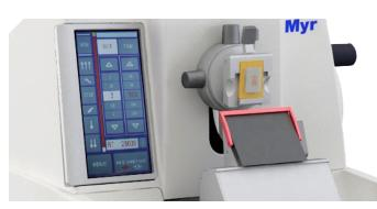
Equipped with a **specimen orientation head** that works with different specimen clamp types and an easy-to-operate change system thanks to the blocking mechanism. Indication of 0-position in x and y direction by palpable click for the precise position of the specimen. Cutting-edge design of the specimen clamp that prevents building up of dirt and facilitates operations with the microtome.
